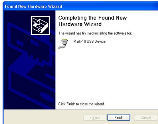
Click "Finish". The Mark-10 USB device is now installed and ready to use. The COM port number assigned by Windows may be identified in Device Manager, or in the communication application being used, such as MESURgauge or HyperTerminal.
